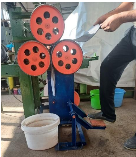
8-rasm. Ko‘p operatsiyalili valli texnologik mashinaning stendi (UzR FA MINSMI)
