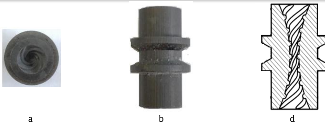
3-rasm. Ichki yuzasi giperbola shakldagi spiralsimon refliyalipga soxta buram 4-beruvchi qurilma
