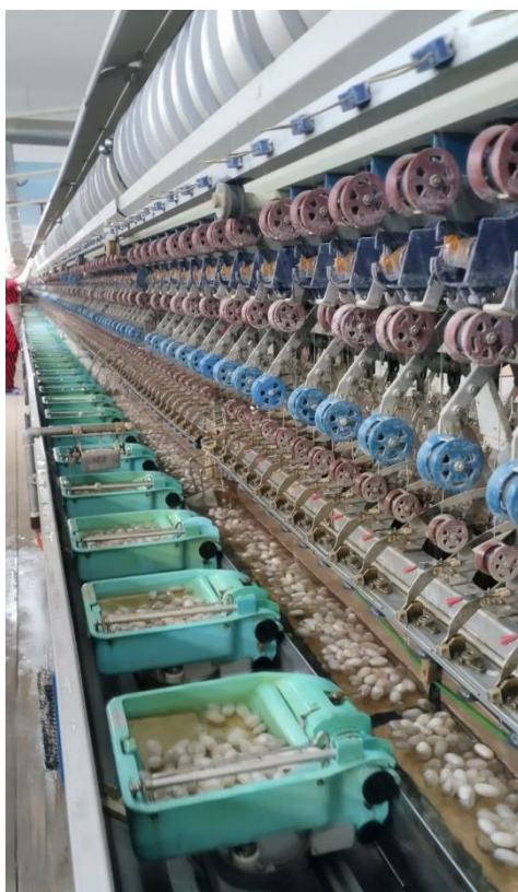
7-rasm. Indigenous automatic reeling machine (IARM) rusumli chuvish dastgohi
