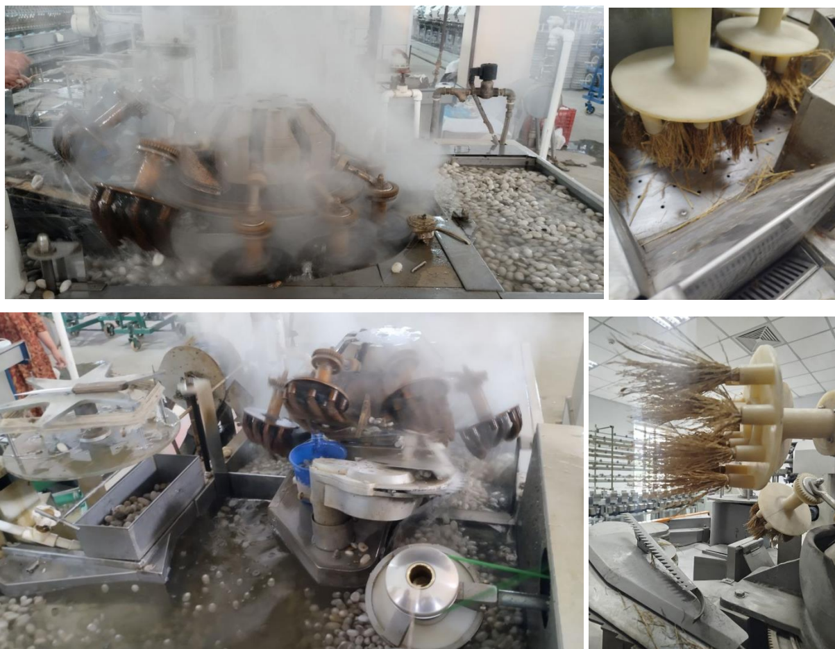
5-rasm. Indigenous automatic reeling machine (IARM) rusumli silkitib yakka uchini topish dastgohi.
