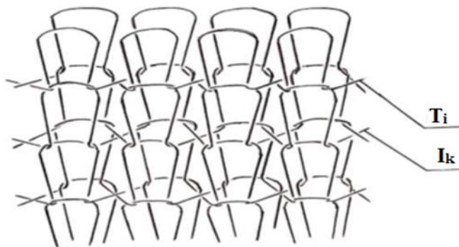
1-rasm. Yangi tuzilishli aralash interlok to'qimasining tuzilishi
