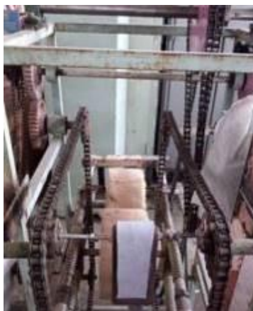
18-rasm. Ko‘n yarim mahsulotini siqish uchun tayanch metall-keramikali tayanch plitali tajriba stendi
