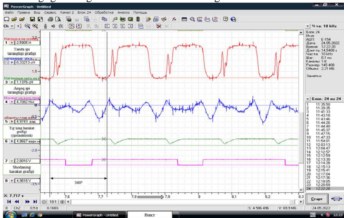
10-rasm. Bazalt iplaridan olovbardosh to'qimani ishlab chiqarishda tanda iplarining taranglik tenzogrammasi
