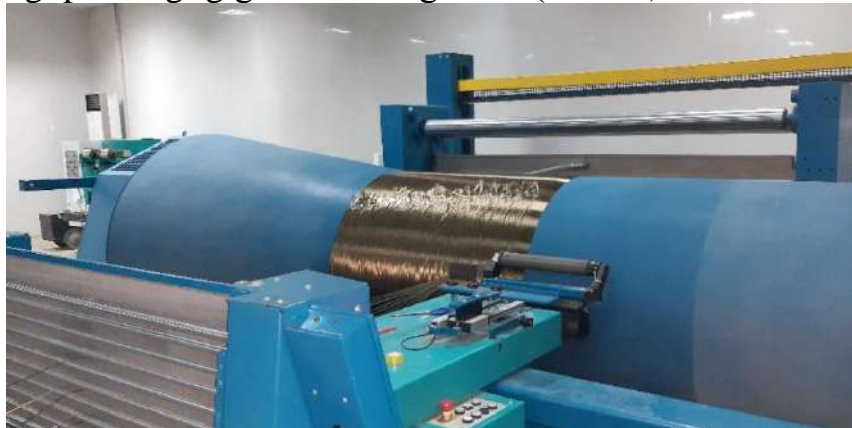
6-rasm. Bazalt iplarini Benninger pitalab tandalash mashinasida tandalash
