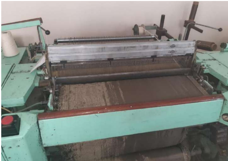
8-rasm. ATPR to‘quv dastgohida bazalt to‘qimasini to‘qish
