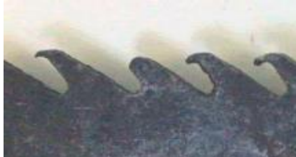
2 - rasm. Jin arralari tishlarining sinishi
