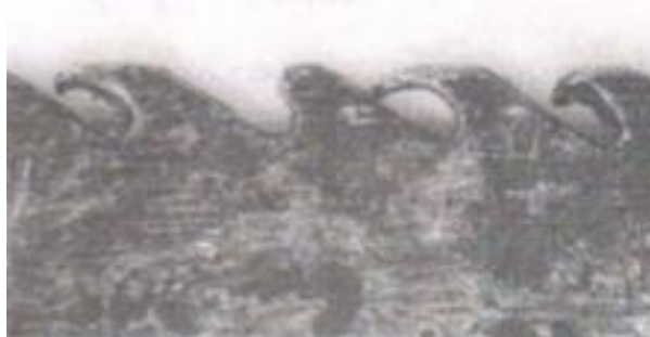
1 - rasm. Jin arrasi tishlarining plastik ezilishi natijasida tishlar
