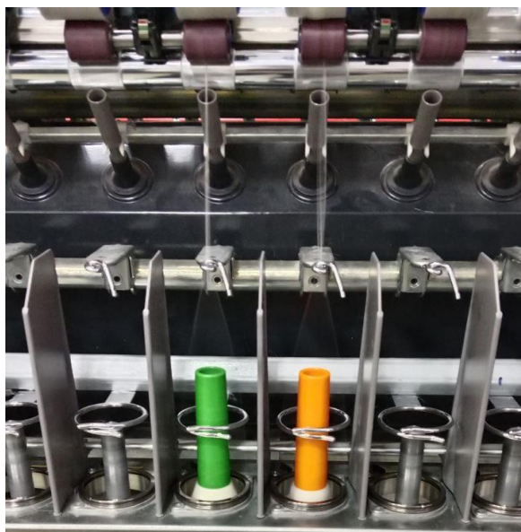
2-rasm. Halqali yigirish mashinasida ip yigirish jarayoni
